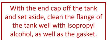
Lay the gasket out gently, lining up all the holes of the gasket with the tank.
