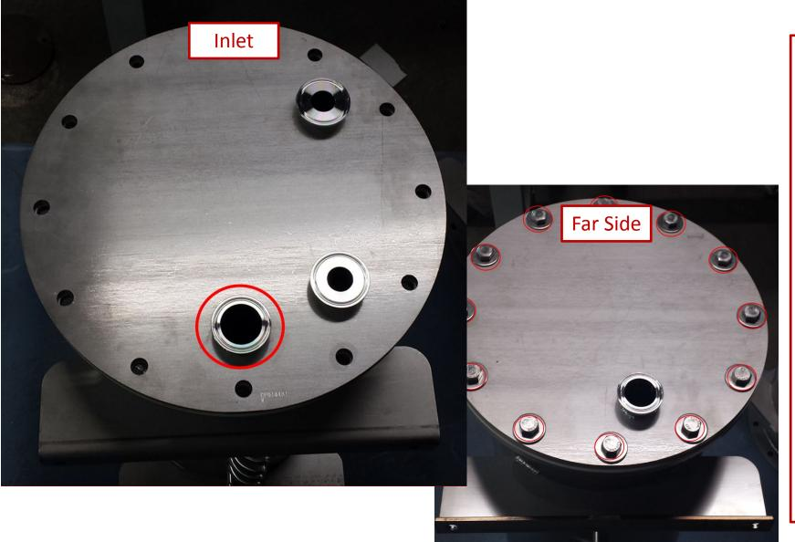
After cleaning the end cap itself with Isopropyl as well, carefully lay it down on top of the gasket with the bolt holes aligned. The gasket likes to slide or shift during this process so do so slowly and gently to make sure everything stays put.
