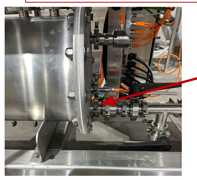
Place the tank back onto the frame but do not tighten down the 4 securing bolts quite yet. We will first make the product inlet connection.
