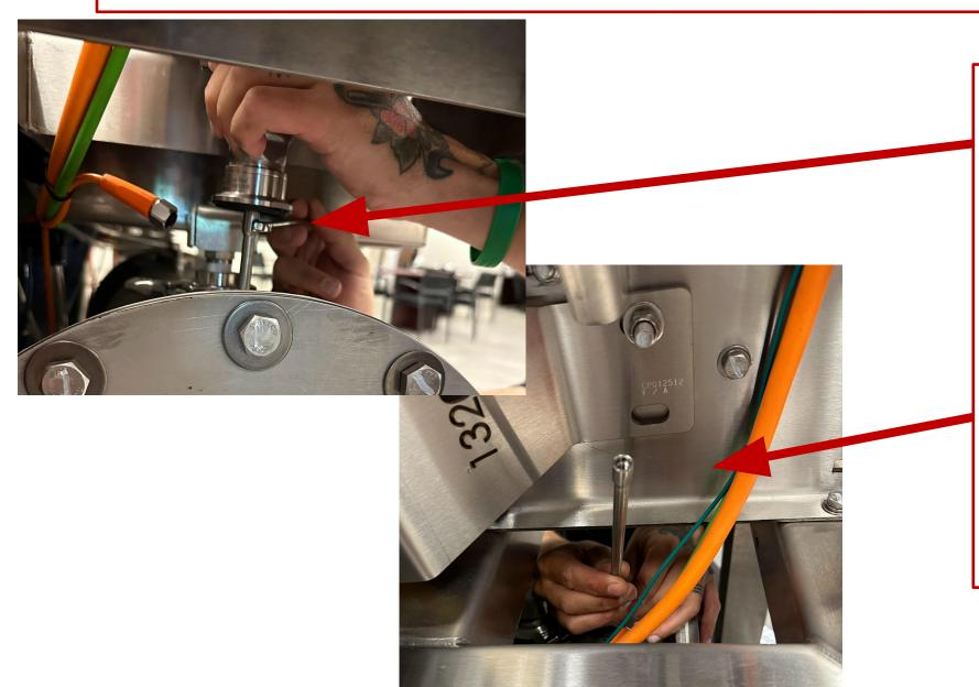
Use an 8mm wrench and remove the spear from the unit by turning the spear counter clockwise unscrewing it from the sensor body.
