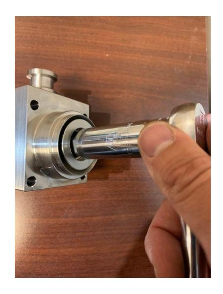
Using a %" Socket Wrench, loosen the Float Claw & Ball assembly and remove it from the Centering Bell Stem.
