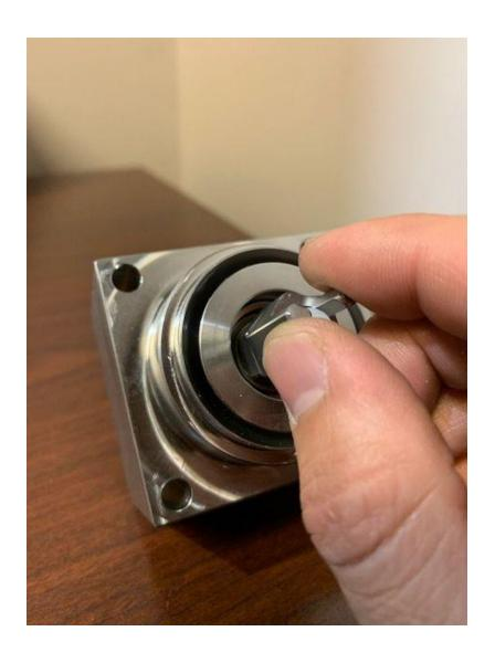
Thread the Float Ball & Claw assembly back onto the Centering Bell Stem by hand.
