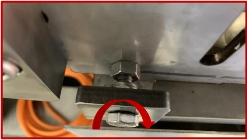
Turn the end positioning bolt head to the right to pull the screw towards the discharge
