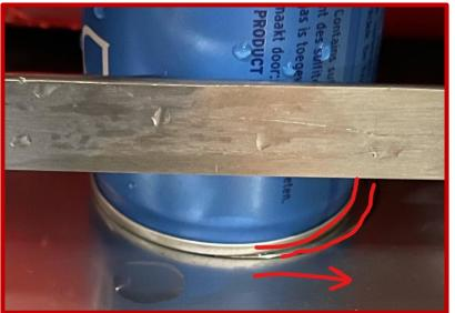
This particular screw, on a Right Hand Filler, needs to move towards the outfeed of the seamer.
