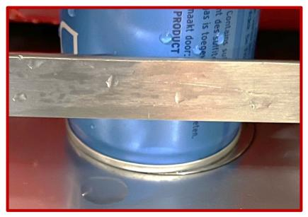
Now, gently push the can from the base into the back of the dwell and evaluate the positioning of the screw. Ideally the can should land dead center on the lifter pad.
