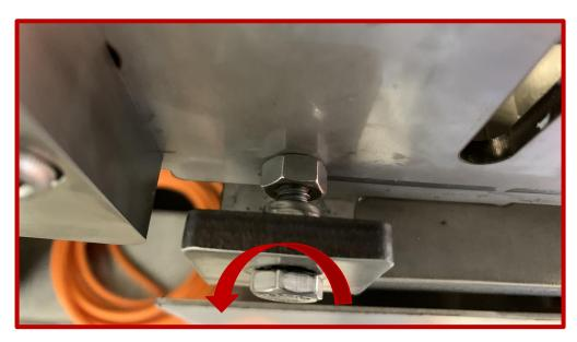
Turn the end positioning bolt head to the left to push the screw towards the filler
