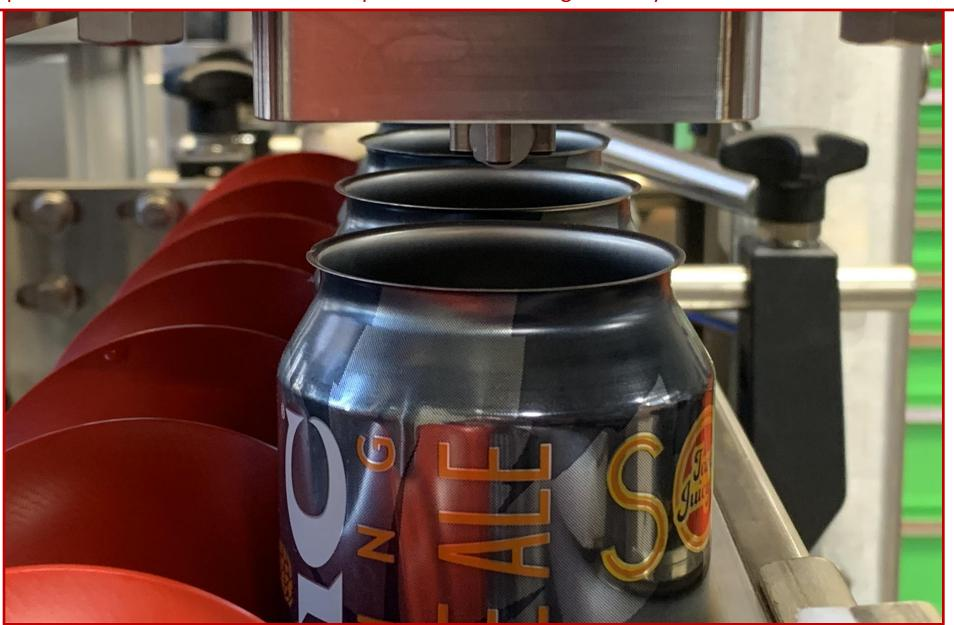
Adjust each side of the index screw until the cans are centered depth wise underneath the fill heads when looking down the row of cans. As the adjustment is made ensure the cans are gently pushed into the back of the screw pocket. The siderails may need to be opened if adjusting forward
