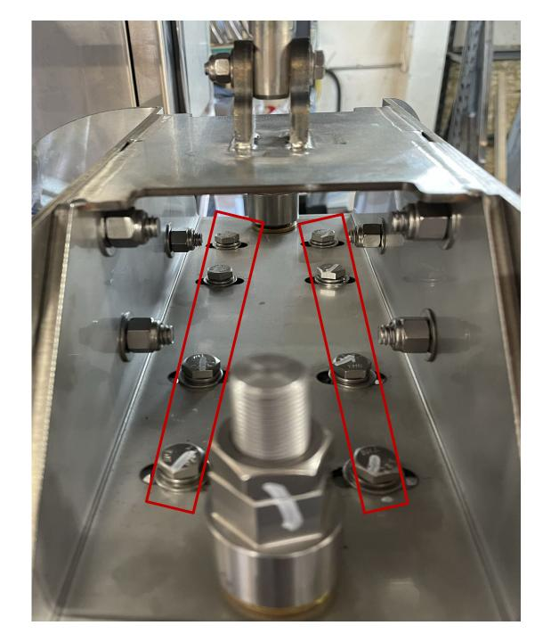
If you are resetting the entire section, start by centering your fill head carriage. The upper bolts securing the fill head actuators are centered at the factory and are very rarely adjusted, especially when talking about can alignment. Alignment is set below the fill head carriage by using the adjustment points we will point out in this walk through as we go forward.
